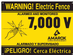
WARNING SIGNS SHALL BE PLACED AT EACH ENTRANCE OF THE PROPERTY AND 30 FEET ON CENTER THEREAFTER EXAMPLE WARNING SIGN @ 9"x12"
