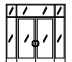
A. KAWNEER AA 425 SERIES FOR FOIL ALUMINUM STORE FRONT OR GLASS DOORS WITH FULL LIGHTS & GLASS
