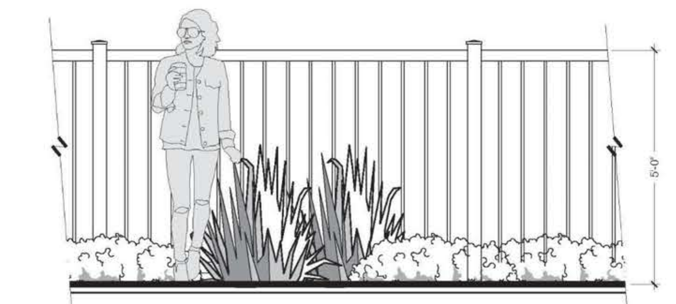
C 5' HT. TUBE STEEL POOL ENCLOSURE SCALE: 1/2" = 1'-0"
