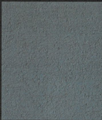
3-COAT STUCCO SYSTEM MANUFACTURER: - PROFILE: ACRYLIC MEDIUM SAND FINISH COLOR: BLDG DB GRAY LIGHT
