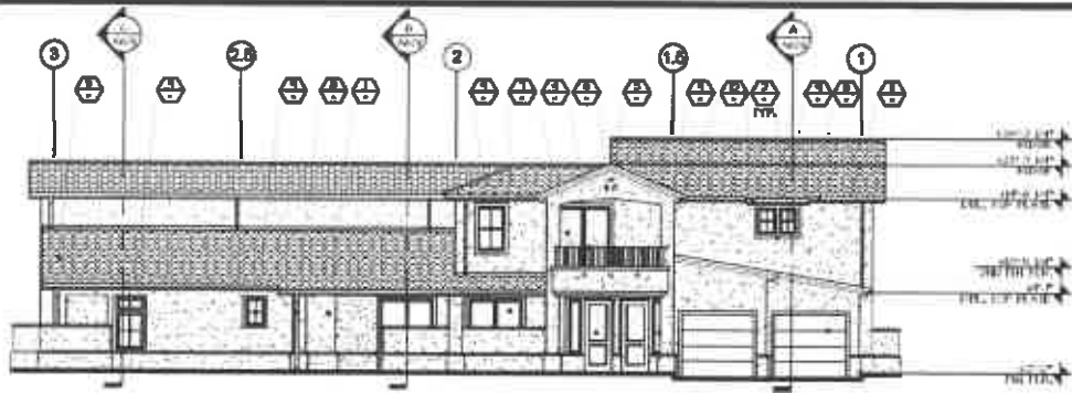
A BUILDING A - FRONT ELEVATION
