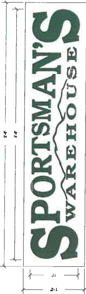
3 POLYCARBONATE FACES WITH VINYL GRAPHICS SCALE: 1/12" = 1'-0"
