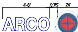
15" ARCO channel letters with 24" Spark FOR USE WITH FASCIAS 18" TO 23" ARCO letters must be positioned to the left of the Spark
