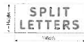
FIGURE 17.48.070(A)(2): MEASUREMENT OF SIGN AREA
