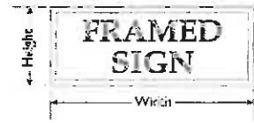
FIGURE 17.48.070(A)(2): MEASUREMENT OF SIGN AREA
