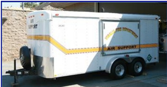
Air Support Trailer - Housed at Station 51 and is used to re-fill SCBA tanks for all Stations. The Trailer is mobile and can be transported to scenes to fill bottles on long term incidents. It has its own generator to be self-sufficient at scenes or can be plugged into station electrical.
